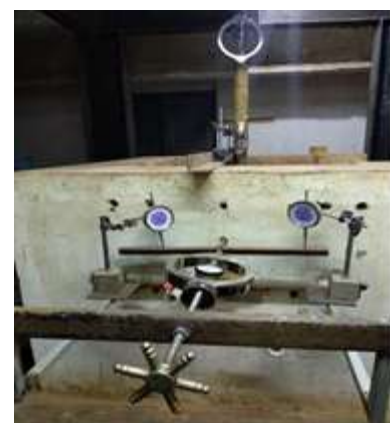
Fig. 3 Arrangement for Lateral loading
