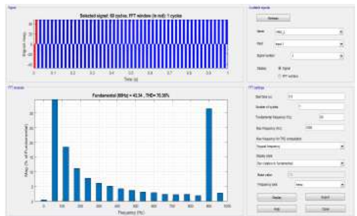
Fig -11: THD for conventional inverter voltage output.
