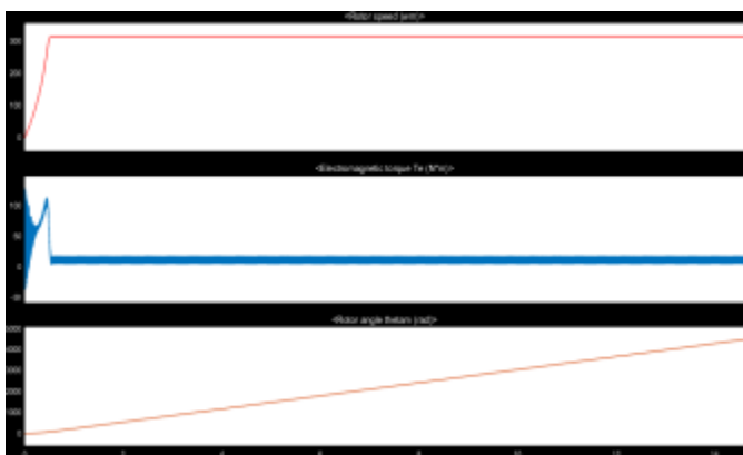
Fig -19: Output torque and Speed for Five level Diode clamped multilevel inverter.
