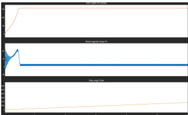
Fig -18: Output torque and Speed for Three level Diode clamped multilevel inverter.
