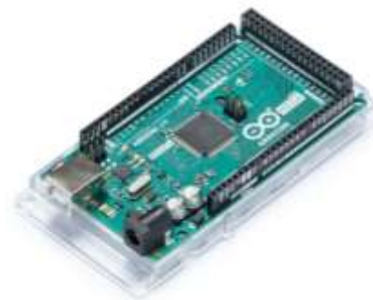
Fig-2: Arduino Mega board with ATmega2560 microcontroller
