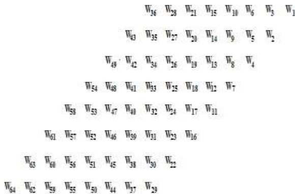
Fig-3: Partial Product of Multiplication for any 8-Bit Multiplications
