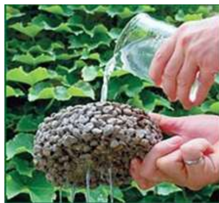
Fig.1: Seepage of water through Permeable Concrete
