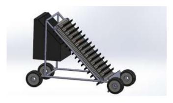
Design of beach sand cleaning machine is done in "Solid works". Dimensions are 600mm length, 500mm hight, 300 mm width and 250mm working width.
