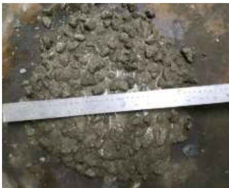
Fig-3: Flow Table Test
