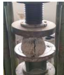
Fig-5: Split Tensile Test on Cylinder
