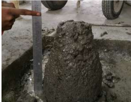
Fig-2: Slump Cone Test
