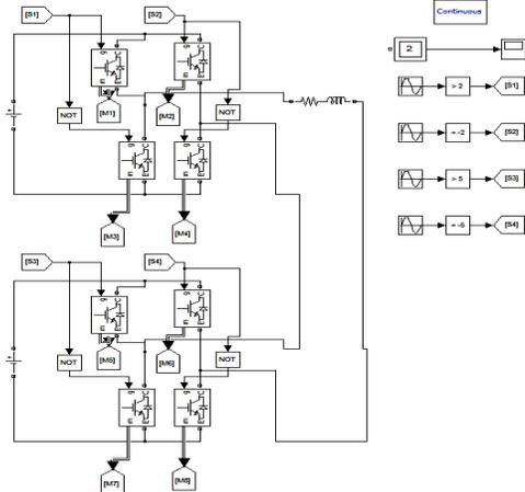
Fig 12 schematic Simulation circuit of a five-level inverter
