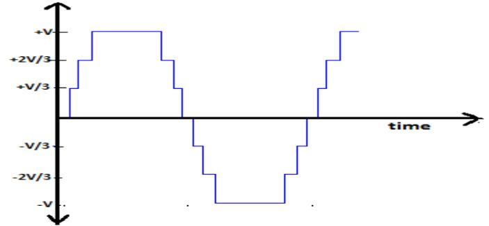
Fig 7 output voltage waveform of a seven-level inverter
