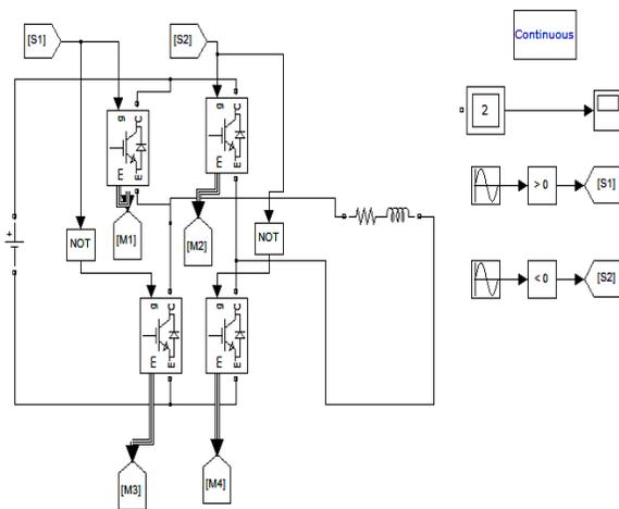
**Fig 8 schematic simulation circuit of a two-level inverter**
