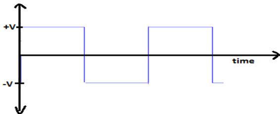
Fig 2 voltage waveform of a two-level inverter
