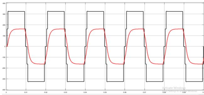
Fig 13 Output voltage waveform and current waveform of a five-level inverter.
