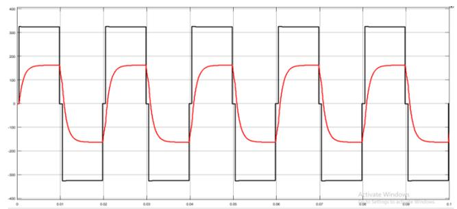
**Fig 11 Output voltage waveform and output current waveform of a three-level inverter.**
