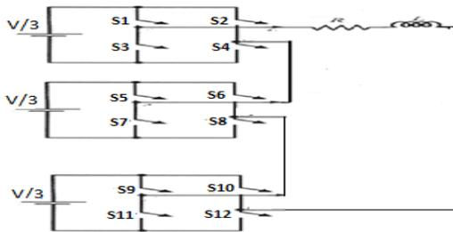
Fig 6 schematic circuit of a seven-level inverter
