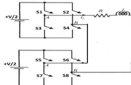
Fig 4 schematic circuit of a five-level inverter
