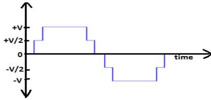
Fig 5 output voltage waveform of a five-level inverter
