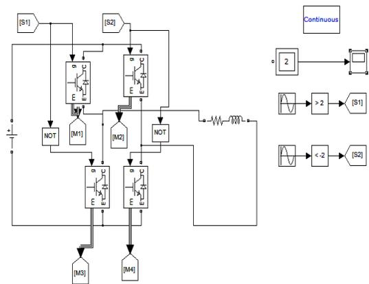
**Fig 10 schematic Simulation circuit of a three-level inverter**
