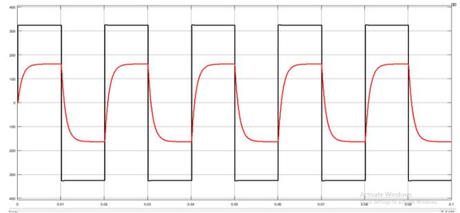
**Fig 9 Output voltage waveform and output current waveform of a two-level inverter.**
