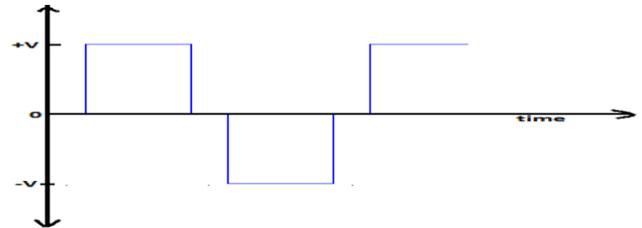
Fig 3 voltage output of a three-level H bridge inverter
