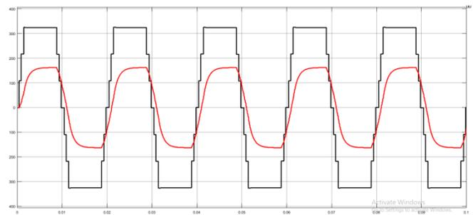
Fig 15 Output voltage waveform and current waveform of a seven-level inverter.
