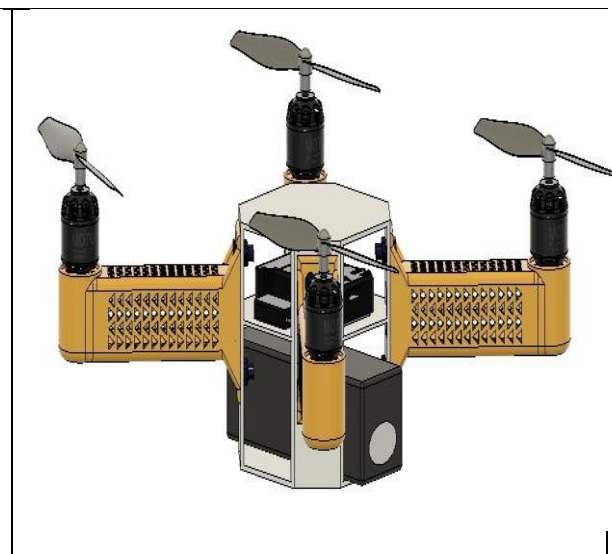
Figure 2. CAD model of a completely assembled quadcopter
