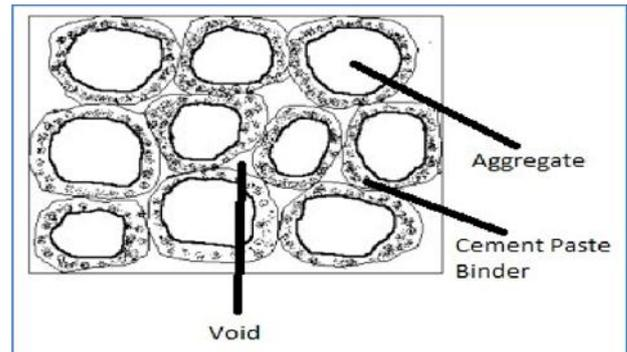
Figure 1 Pervious concrete diagram
