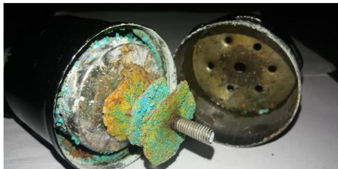
Set-up having \text{ZrO}_2 coated cylinder & \text{CuSO}_4 coated nets
