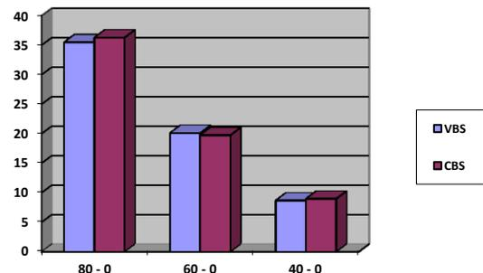
Hence, a vehicle equipped with this system i.e. VBS is capable of reducing the braking distance, when traveling at 80 kmph, from 36.30 meters to 35.50 meters.
