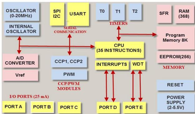
Fig -2: Architecture of PIC18
