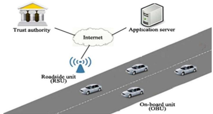
Fig.2. System Architecture.
