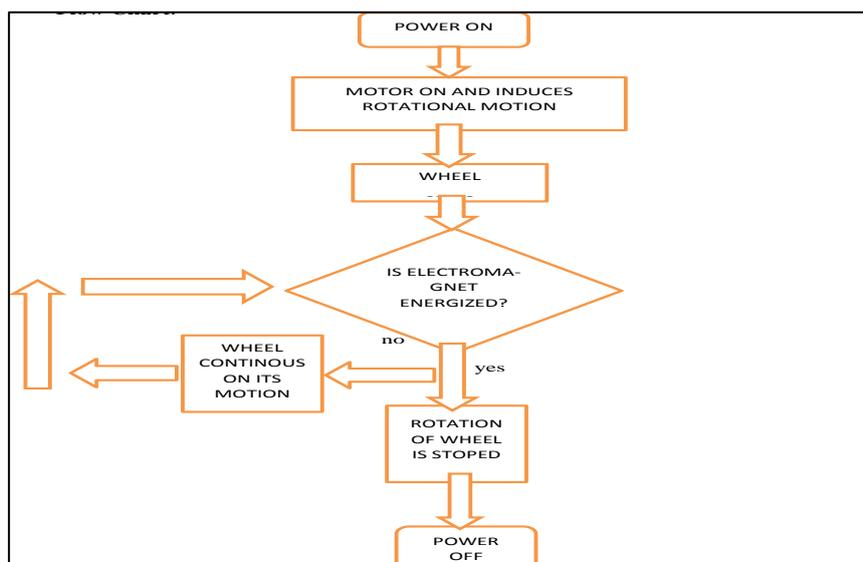
Figure1. Flow Chart for Working of Electro Magnetic Brakes
