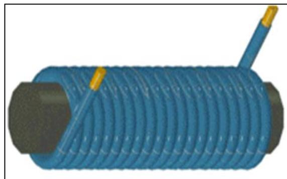
Figure 5. Electromagnet
