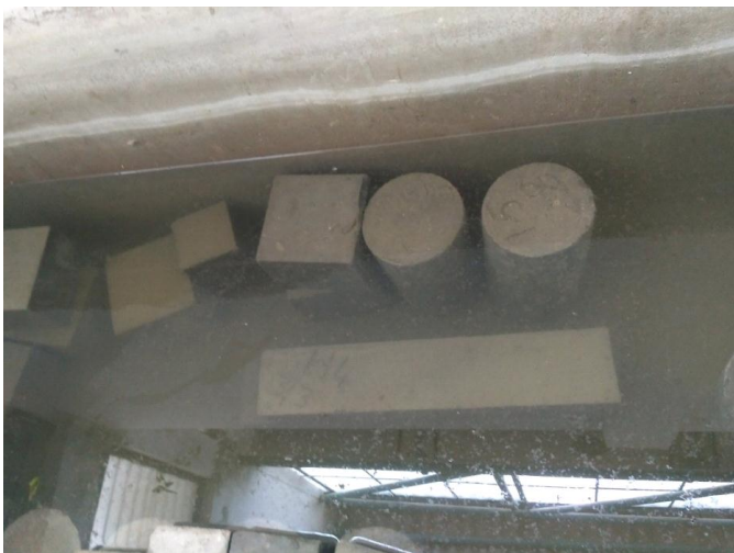
Fig 5 Curing of concrete moulds
