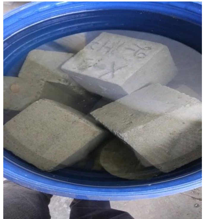
Fig 2 Curing of specimens for chemical attack test
