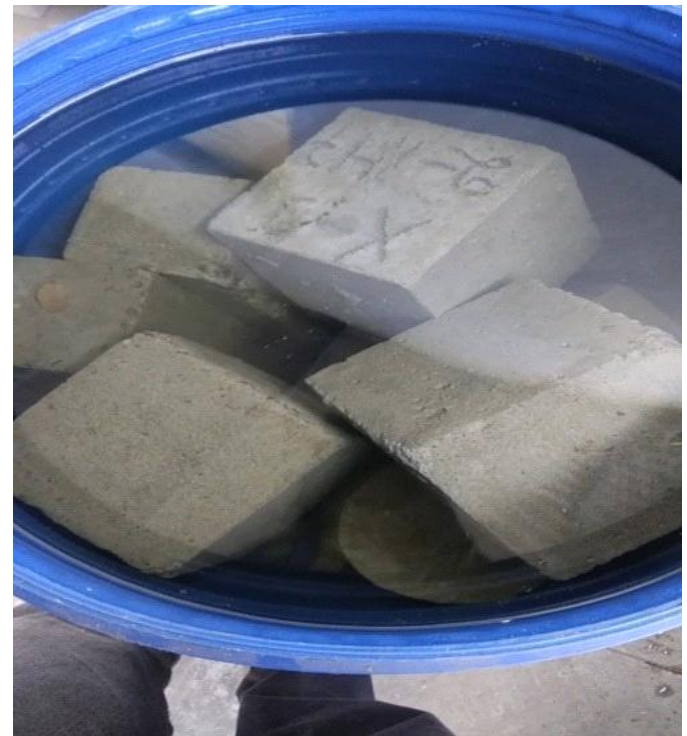
Fig 2 Curing of specimens for chemical attack test
