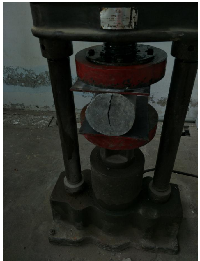
Fig: 3 Split tensile strength of concrete
