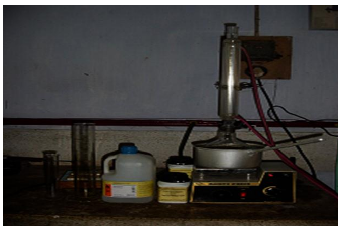
Fig-3: Instrument used for the Transesterification process
