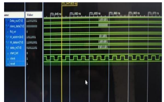
Fig. 14 Slave 8-piece data transfer to master
