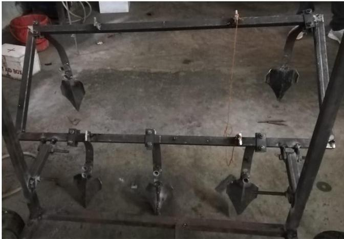
Fig. 4.7 Ploughing Tool and Frame
