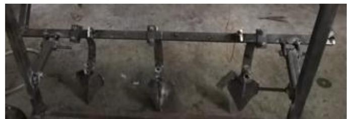
**Fig. 4.2** Actual fabricated Plough
