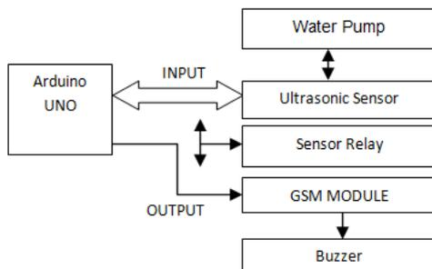
Fig -2: Block Diagram for monitoring system using GSM model
