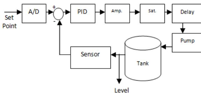
Fig -1: Block Diagram for PID controlled monitoring system
