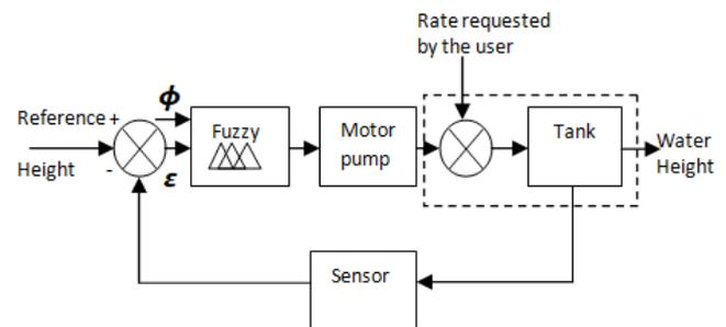
Fig -3: Block Diagram for monitoring system using Fuzzy Logic
