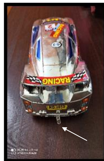
Fig -4: Receiver module at tail-light of the vehicle
