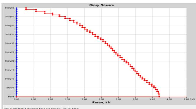
Figure 9.2.2 Base shear RSY dynamic Analysis for Structural wall and Moment frame
