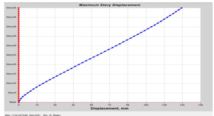
Figure 9.3.1 Lateral Displacement RSX dynamic Analysis for Structural wall and Moment frame
