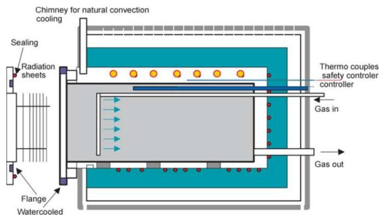
**Figure 6** Internal structure of Muffle Furnace
