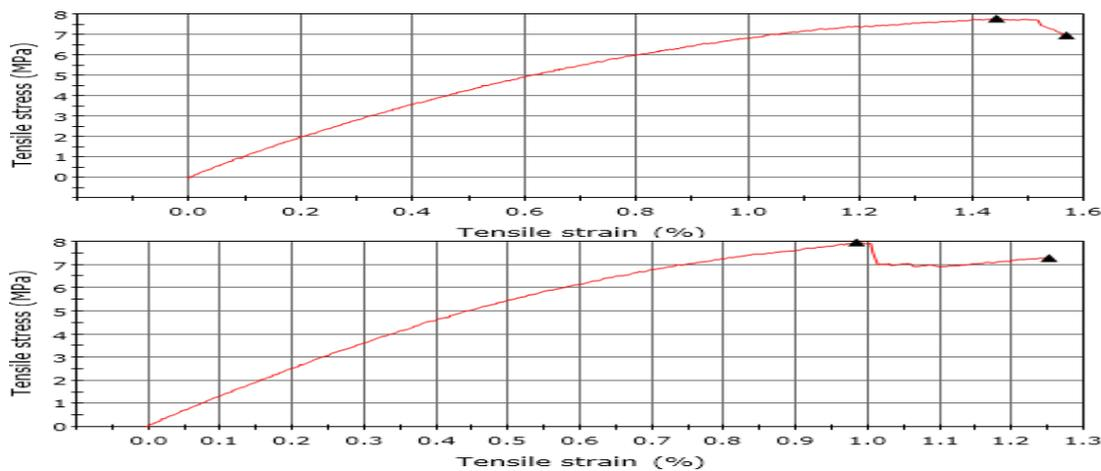
Figure 8 Tensile stress vs Tensile strain (without metal)
