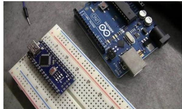
Fig-4: Arduino Nano and Uno
