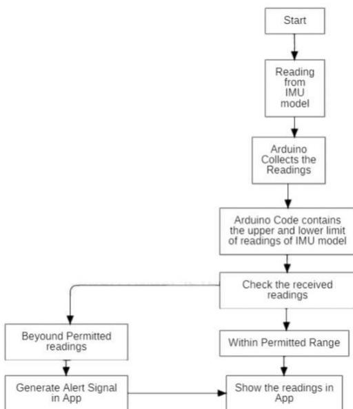
**Fig-1:** Flowchart of Posture detection and correction device
