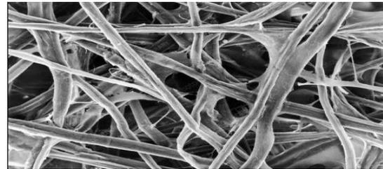
**Fig 5: Cellulose fibres**
