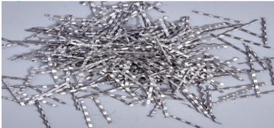
**Fig 3: Steel fibre**
