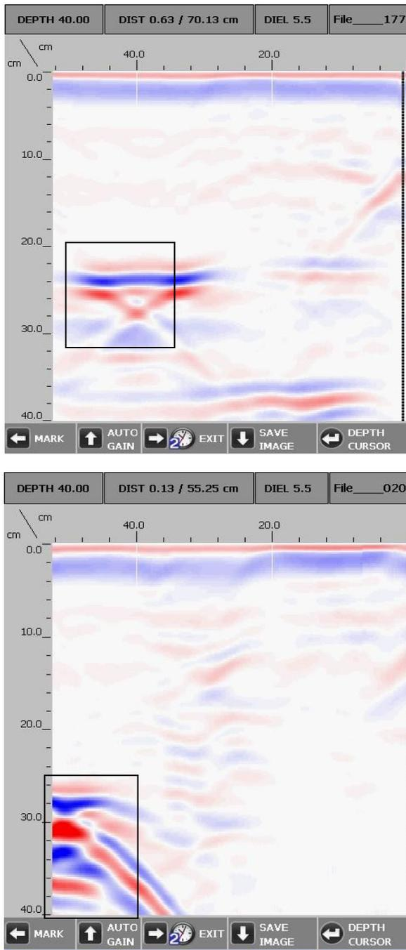
**Fig-2:** scanned data (radargram) of voids in perpendicular dimension.
