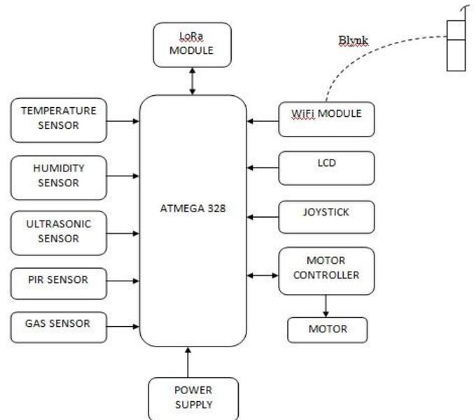
Fig -2: Block Diagram of Proposed Prototype
