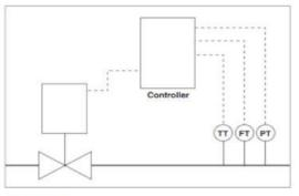
Transmitters: Flow (FT) Temperature (TT) Pressure (PT)
