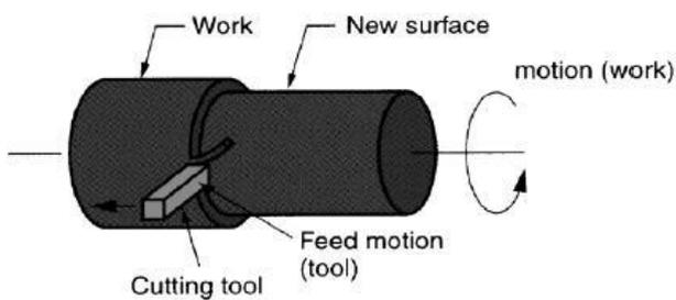
Fig.2. Turning operation [40]
