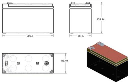
**Fig-10: Battery of Vehicle**
