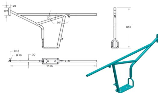
Fig-6: Main Frame of Vehicle
