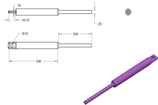
Fig-7: Wheel clamp of Front wheel
