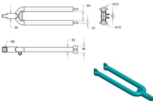
Fig-5: Wheel Clamp at Bottom rear
