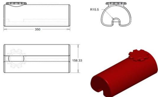
Fig-8: Fuel Tank of Vehicle
