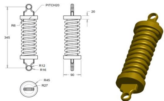
**Fig-2: Suspension of Vehicle**
