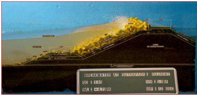
**Figure 2: Wave action on armor layer of breakwater consisting of 12 t tetrapods at -8.0 m bed level with +4.73 m water level and 5.8 m wave height**
