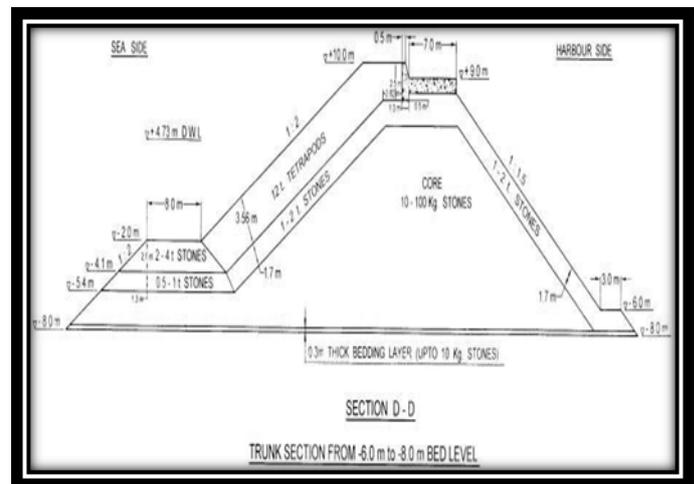
**Figure 1: Cross-section D-D trunk section from -3.0m to -6.0m bed level of breakwaters for the proposed development of fishery harbor at, Gujarat.**
