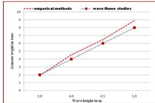
**Figure 3: Armor Weight V/S Wave Height**
