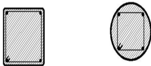
Fig.3 Concrete filled steel tubes (CFST)(rectangular and circular sections)
