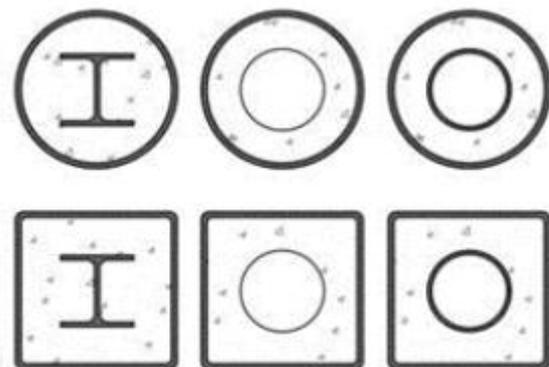
Fig. 4 Combination of CES and CFST, hollow CFST section and double skin sections Preetha et al., [2]
