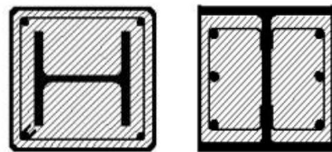
Fig.1 Fully concrete encased steel column Fig.2 Partially concrete encased steel (CES) column
