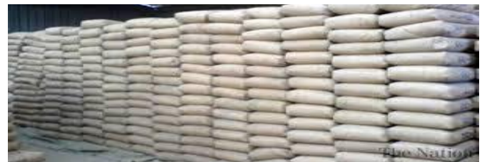
Premixed mortar should be stored in closed shed with elevated platform, covering with tarpaulin to avoid touching with soil and moisture.
