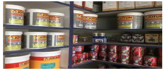
Painting materials should be kept on raised platform, in rack with proper segregation and identifications for easy handle and inventory.
