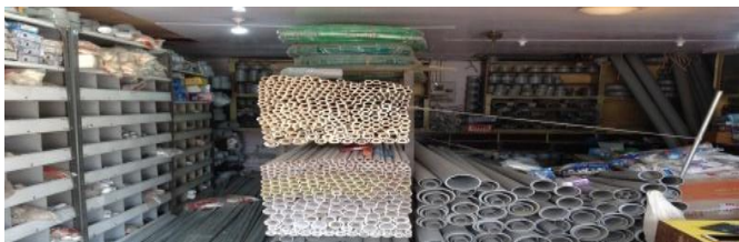
Plumbing materials and its fittings should be stacked on racks with proper segregations as per specifications for easy access and inventory control.
