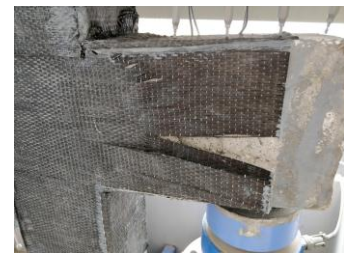
Photograph -7: Failure pattern observed in case of CFRP2 specimen
