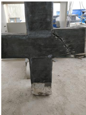
Photograph -4: Front face, Back face and Side face pattern of FRP fabric
