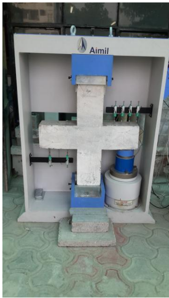
Photograph -3: Experimental set up with locations of LVDT
