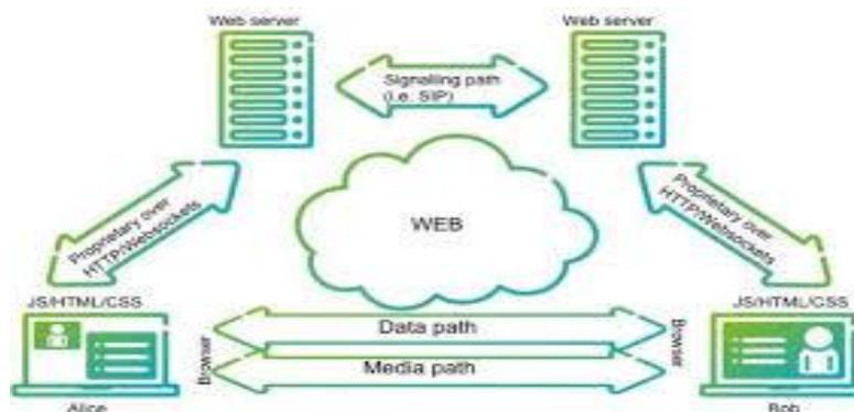
Fig-1 Architecture of WebRtc
