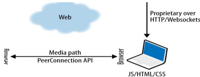
Fig-2 WebRTC Signaling Mechanism
