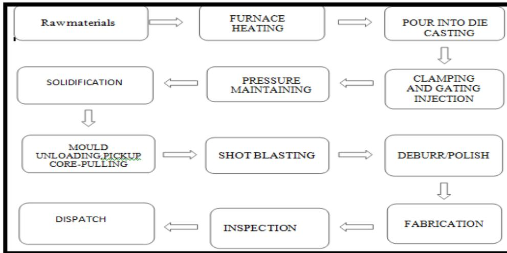
Fig- 3. Process flow of Pressure Die Casting
