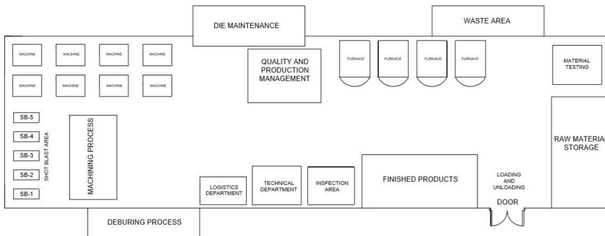
Fig - 2. Optimized Layout of Pressure Die Casting Process
