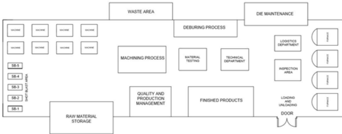
Fig - 1. UnOptimized Layout of Pressure Die Casting Process.
