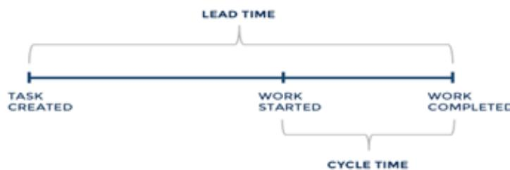
Fig- 4. Lead time and Cycle time
