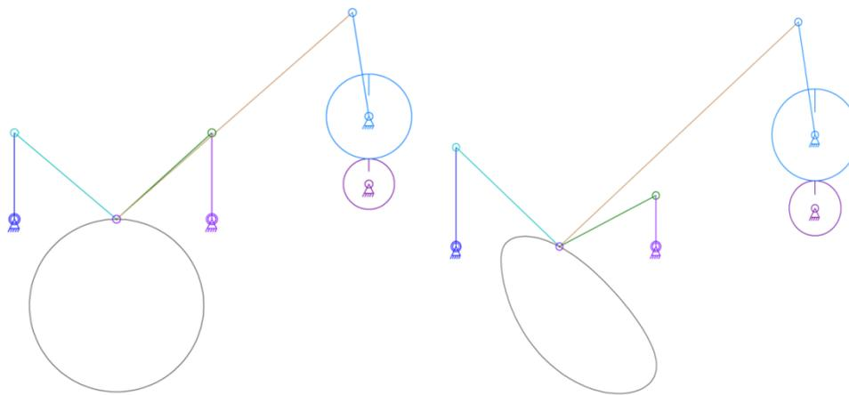
**Fig. 4 Eight Link Gear Mechanism in Configuration IV and Possible Coupler Curves**
