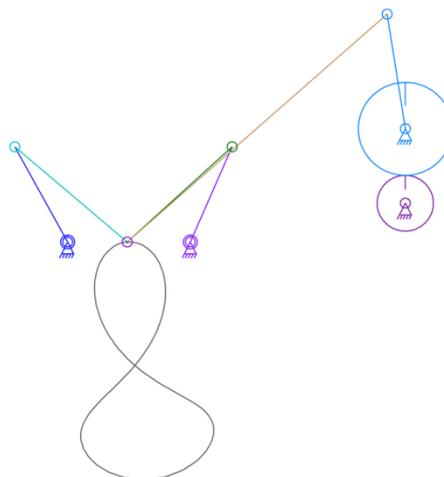
**Fig. 3 Eight Link Gear Mechanism in Configuration III and Possible Coupler Curve**
