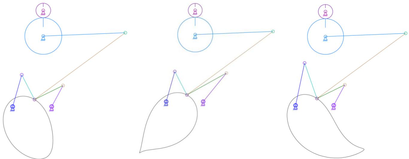
**Fig. 1 Eight Link Gear Mechanism in Configuration I and Possible Coupler Curves**
