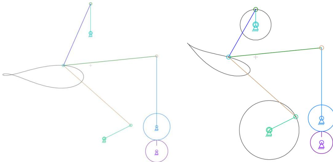
**Fig. 8 Eight Link Gear Mechanism in Configuration VIII and Possible Coupler Curves**
