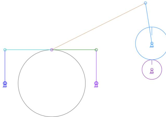
**Fig. 6 Eight Link Gear Mechanism in Configuration VI and Possible Coupler Curve**
