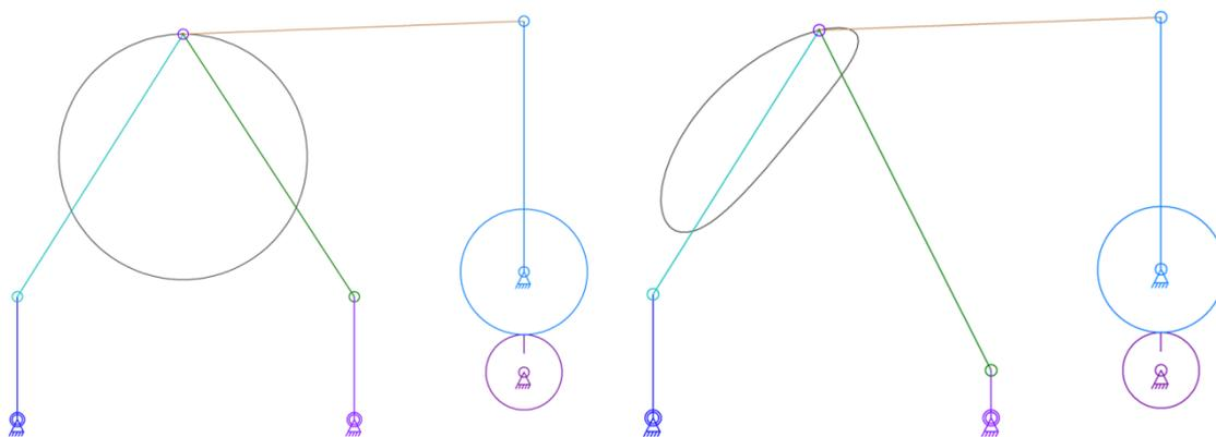
**Fig. 7 Eight Link Gear Mechanism in Configuration VII and Possible Coupler Curves**
