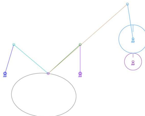
**Fig. 5 Eight Link Gear Mechanism in Configuration V and Possible Coupler Curve**
