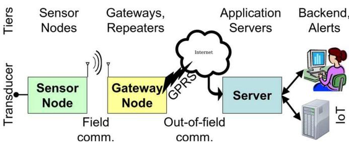
Figure 8 Tiered structure of the WSN platform.
