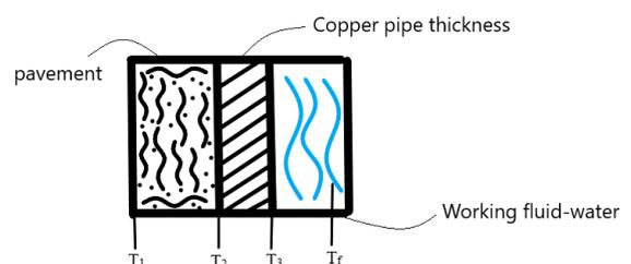
Here,  $T_1$  = Temperature of base layer of pavement =  $60^\circ\text{C}$
