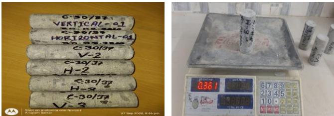
Fig-2: Extracted core specimens & measuring weight of the specimens.
