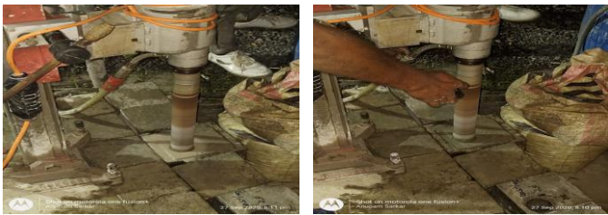
Fig-1: Extraction of core specimens from cube samples.
