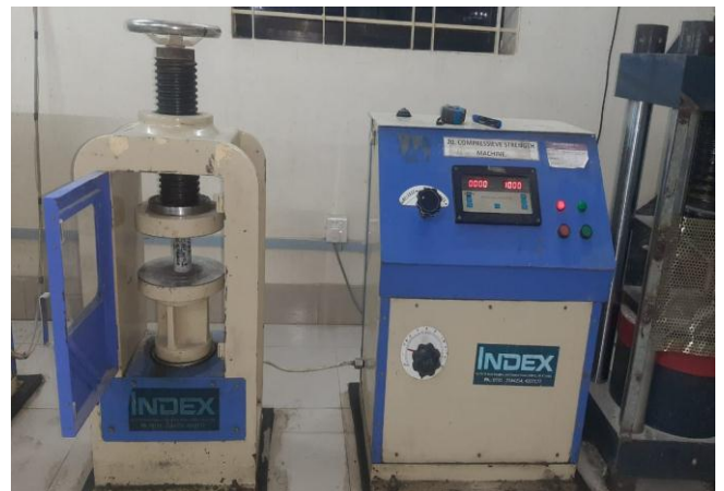
Fig-3: Testing of core specimens for evaluation of compressive strength of concrete core specimens.
