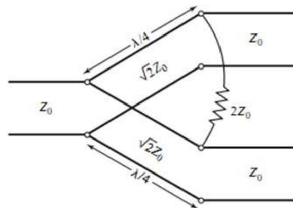
Fig 2(b): Equivalent Circuit of Conventional Power Divider Network
