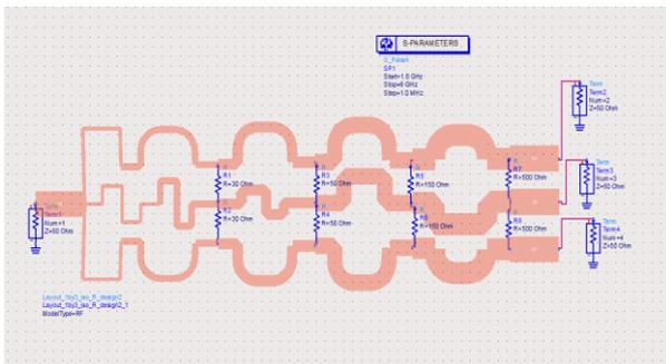
Fig 3: Proposed wideband Wilkinson power divider (WPD). Multi section chebyshev matching network
