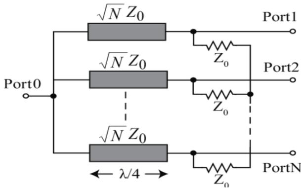
Fig 2(c): N-Way Power Divider for Equal Power Split
