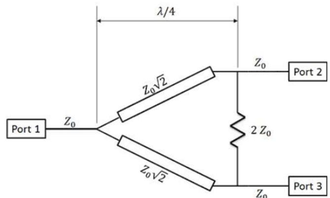
Fig 2(a): Equally-Split 2-way Wilkinson Power Divider
