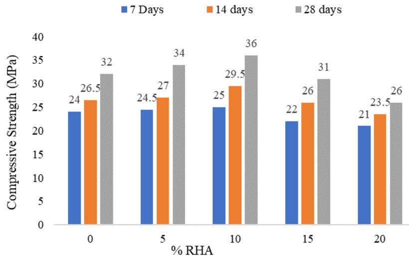
Fig. 3 Compressive strength test results at 7,14 and 28 days [62]
