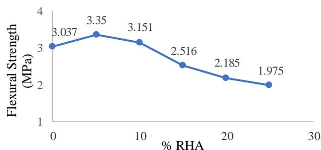
Fig. 7 Flexural strength results at 28 days [60]
