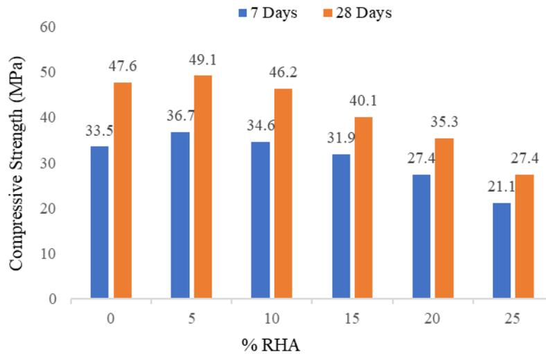
Fig. 1 Compressive strength test results [60]
