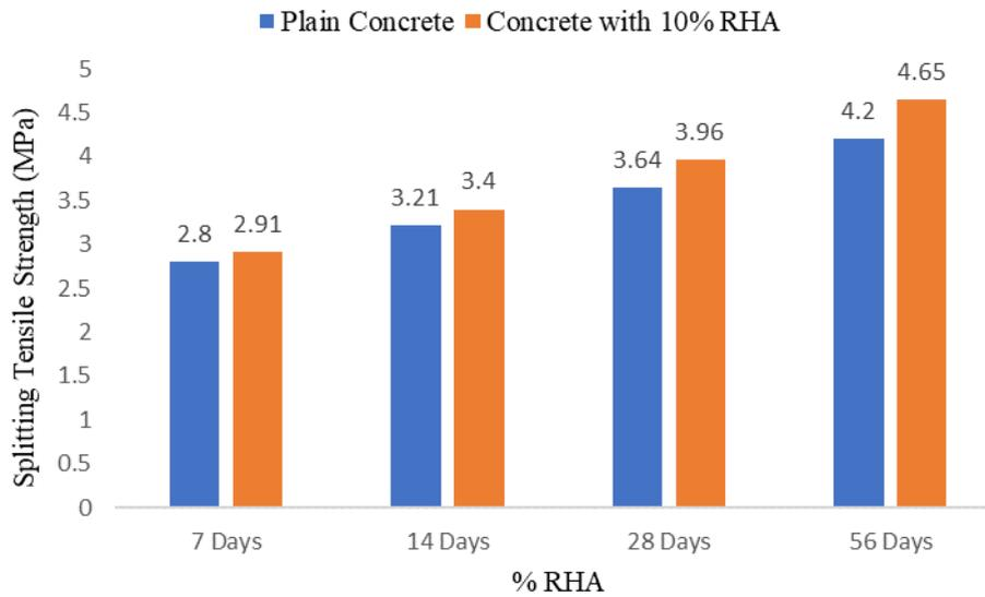
Fig. 5 Split tensile strength of plain concrete and RHA concrete [61]
