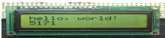
Fig 6. Liquid Crystal Display showing the programmed display after switching it on.
