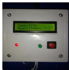
Fig 7a. LCD display of Heartrate and Body temperature on the fabricated device
