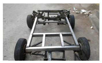
Figure 4.1 Chassis layout.
