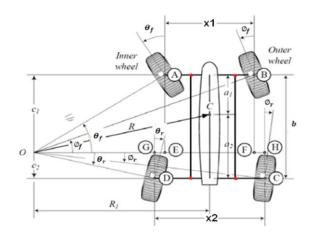
Figure 2.2 Correct Four wheel steering mechanism
