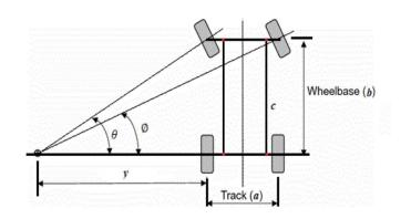
Figure 2.1 Ackermann steering mechanism
