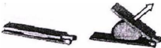
Fig 1: A simple joint based on the expansion principle
