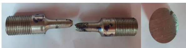
Figure 2.1 Tensile Test Specimen & Figure 2.2 Hardness test on Raw AISI 316L
