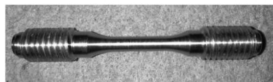
Figure 2.3 Specimen geometry used for fatigue tests.
