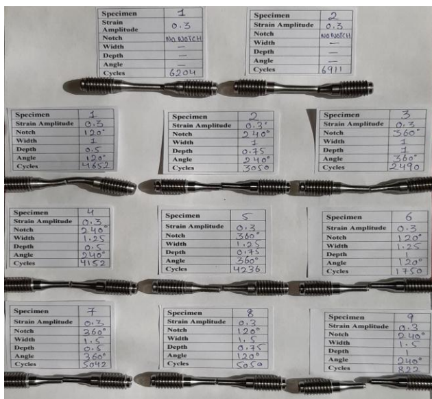
Figure 3.1. Broken specimens with their life cycles
