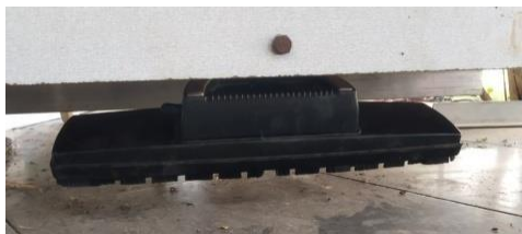
Fig-5: Inlet of the vacuum cleaner at the front bottom
