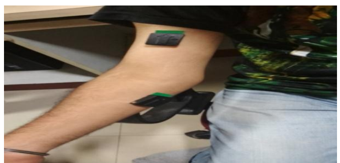
Fig. 9. Sensors on muscles using Double-Sided Adhesive tapes.
