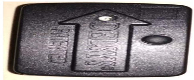
Fig. 6: Wireless sensor used for acquiring EMG.
