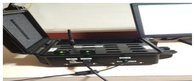
Fig. 8: Trigno EMG wireless system (SP-W02A-1849).
