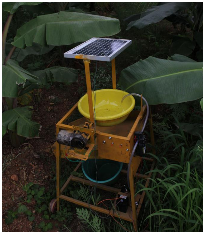
Fig-13: Automated refilling of water to basin
