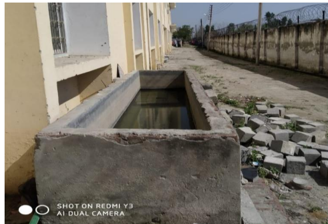
Figure 1 Curing of concrete for 7 days and 28 days
